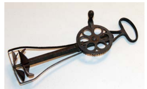
Lyon's Egg Beater & Cream Whip. Patented in 1897. Made in Albany. Features a pair of propellers as part of the mixing mechanism. Each propeller turns in a different direction.
