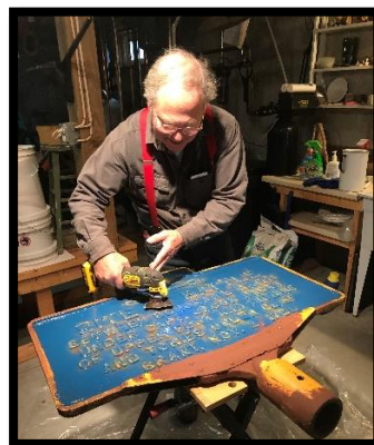
Bob removing the old paint and rust during his repair process.
